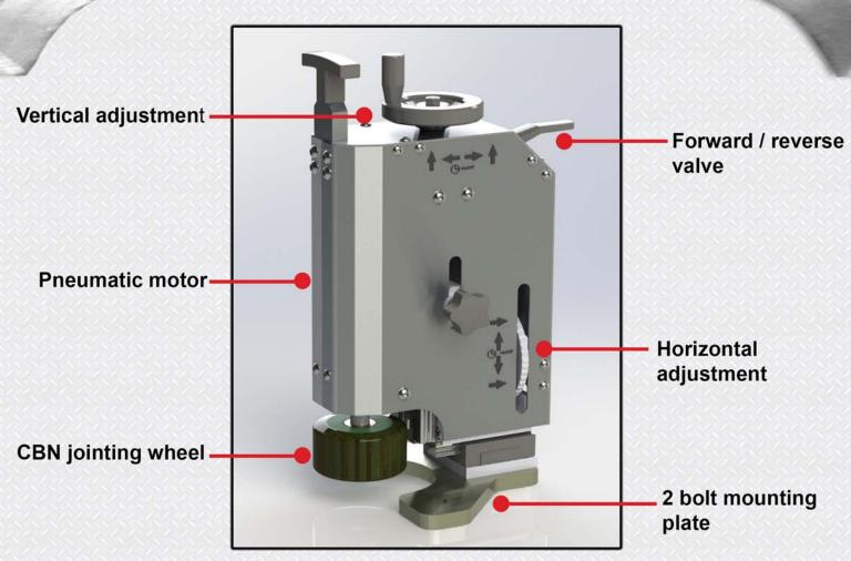
**IMPROVED SAFETY**-jointing occurs when machine is locked out. Safer process vs. traditional jointing because heads are not powered/spinning at 3600 rpm.
