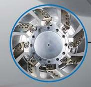
Small head diameters available for small log processors and edgers.
